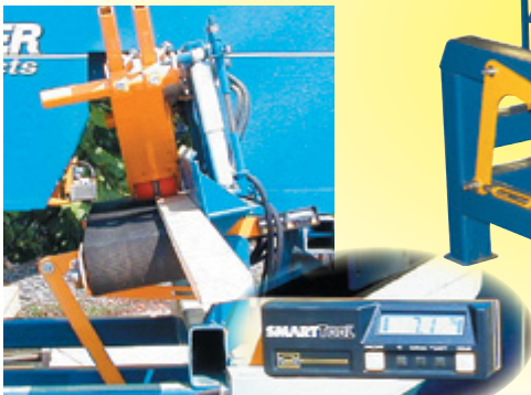
Optional tilting feedworks with extremely accurate degree meter.
