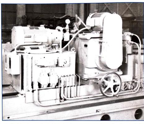
The length of carriage stroke is controlled by two adjustable trip dogs, mounted on the front of the machine base, which actuate a reversing valve on the carriage when the end of the work stroke is reached.
