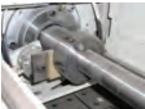
Zero rotation sensor, air actuated brake and door interlock, for safety and reduced down time.
