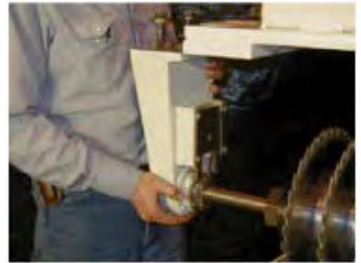
Heavy duty overbeam and cast aluminum slip-off end bearing.
