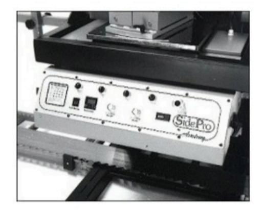
The operator can quickly set the SidePro for right or left hand saws, number of teeth to be side ground and tooth spacing from the control panel.
