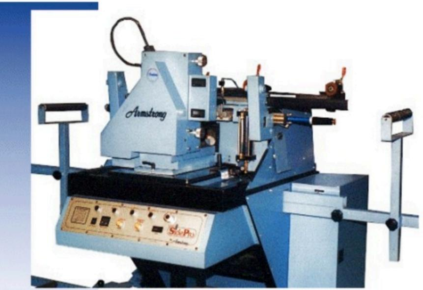
The SidePro's horizontal configuration and dual saw advance system allows both right and left hand saws (or double cut saws) to be accurately side ground in about the same area required for a stretcher roll bench. Note that the digital readouts are conveniently located next to the grinding wheel positioning controls.
